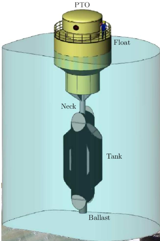
The Waveram is a single-bodied, seaworthy, spar buoy, designed for utility-scale arrays in the most energetic deep-water offshore sites, such as the Atlantic off the West of Ireland and similar ocean sites in the Americas and Australasia.
