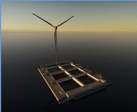
The Blue Growth Farm project, designs an automated, modular and multi-functional infrastructure for open sea installations. During the project development, two scaled prototypes, one (1:40) for indoor (wave tank) testing, and the other (1:15) for outdoor (sea) testing, have been designed and validated by the BGF Consortium at Ecole Centrale (Nantes, FR) and at NOEL (Reggio Calabria, IT), respectively.
