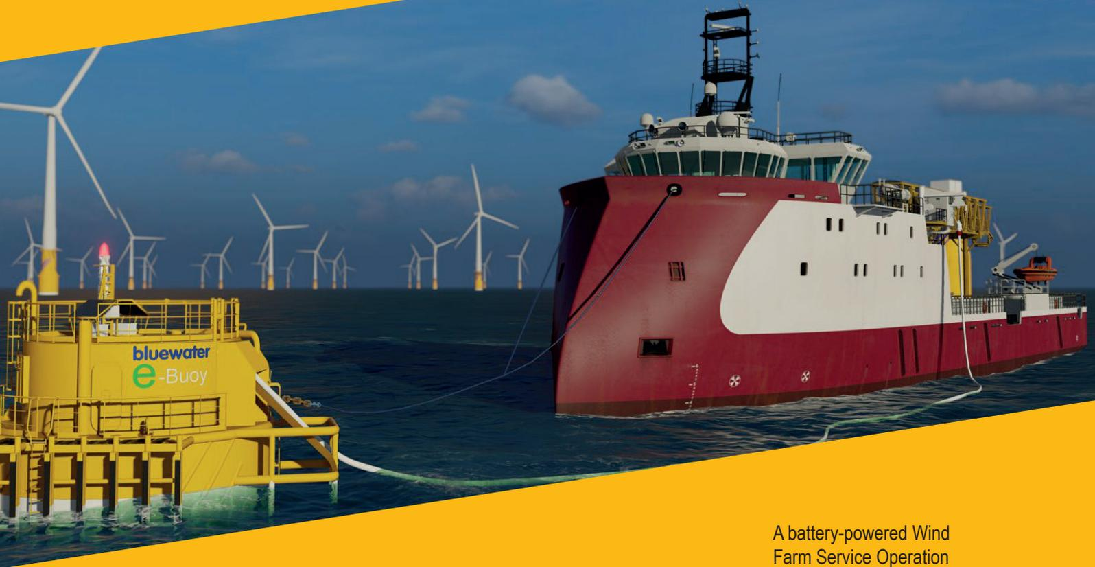
A battery-powered Wind Farm Service Operation Vessel (SOV) receiving electrical power, generated by a wind farm, and transferred by a Bluewater E-buoy. During charging, the vessel is moored to the buoy and power consumption by thrusters is minimized. This concept can assist wind farm operators to meet their Net Zero Carbon targets while ensuring the uptime of their wind farms.
