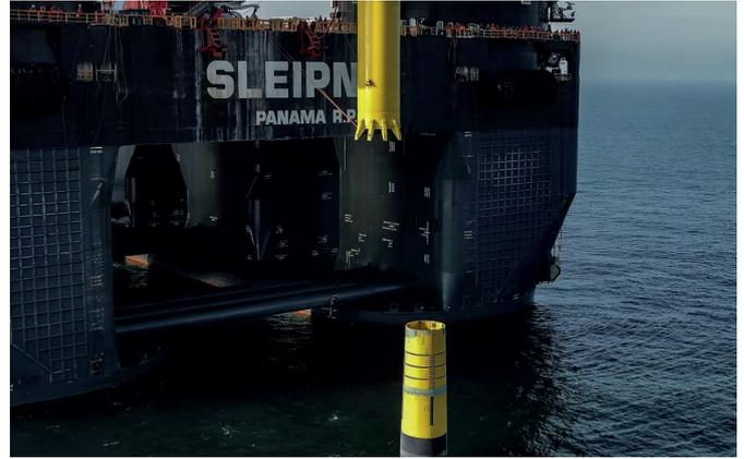
Heerema Marine Contractors has tested its novel Rotor Nacelle Assembly (RNA) installation method offshore for the first time. Heerema performed the demonstration project in collaboration with DOT and the Delft University of Technology (TU Delft) to collect valuable operational data and test installation methods and durations.
