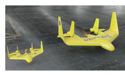
Swedish engineering firm Minesto, a spin-off of Saab, developed a series of tidal turbines, or "sea dragons", that look like submerged aircraft.
